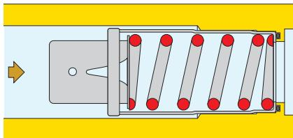
If the differential pressure is within the control range, the piston compresses the spring and gives the medium a free flow area to permit the designated flow to pass.
