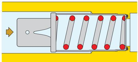
In this case, the regulating piston remains fully out without compressing the spring and gives the medium the maximum free flow area.
