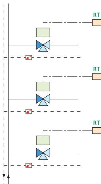
To guarantee the design flow rates (with open or closed valve) to the various zones of a system.
