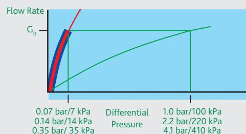
$$Kv_{0.01} = 0.378 \times G_0 \quad \Delta p \text{ range } 7 - 100 \text{ kPa}$$
