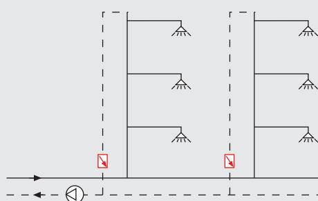
To balance circuits for hot water distribution.
