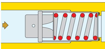
In this case, the piston is fully compressed and only allows flow through the fixed orifice.
