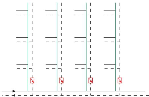
To regulate the flow rate in each riser or secondary branch of a system.
