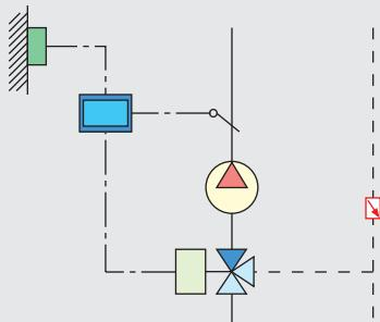
To ensure constant flow rates (in any valve position) in circuits with traditional temperature control.
