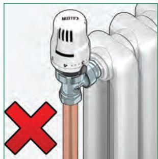
The sensitive element of the thermostatic control heads must never be installed in niches, radiator cabinets, behind curtains or exposed to direct sunlight, otherwise it may produce false readings.
