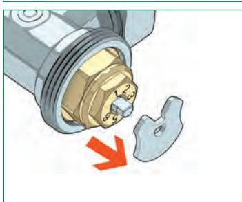
Pre-setting and installation of the thermostatic heads, electronic or thermo-electric actuators
