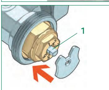
Rotate the control stem to select the desired position.
