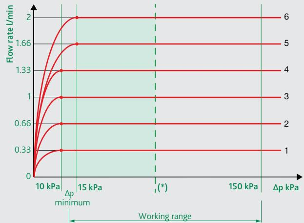
(\*) Recommended working range: for the best dynamic behaviour without problems linked to the passage of the water flow through the valve it is recommended to work with  $\Delta p < 70$  kPa.
