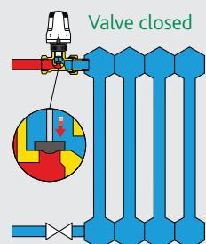
The control device of the thermostatic valve is a proportional temperature regulator, composed of a bellows containing a specific thermostatic liquid.
