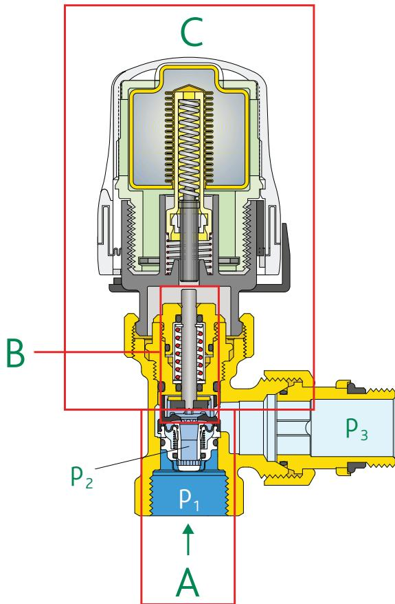
Device (A) regulates the  $\Delta p$  and keeps it constant across the device (B+C), by means of an automatic action (balancing between the force generated by the differential pressure and the internal opposing spring).
