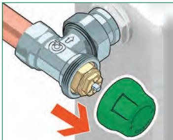
To pre-set the flow rate, position the setting tool on the control stem.
