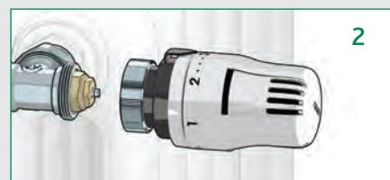
Install the thermostatic (2), electronic (3) or thermo-electric (4) actuator onto the valve.
