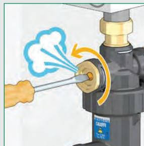
When necessary, it is possible to use the manual air vent in the cap to expel air from inside the strainer.
