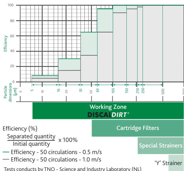
Tests conducted by TNO - Science and Industry Laboratory (NL)
